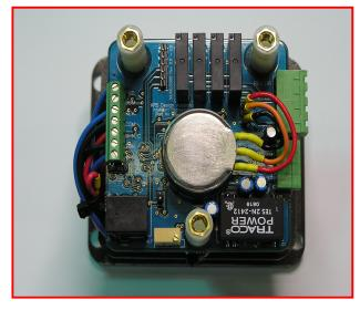
The Footswitch unit is intelligent, with on board microchip that generates all the necessary outputs to drive the machine when the Footswitch is actuated by the driver.
